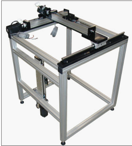
X-Y chemical coating process with open frame aluminum structure
